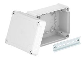
Closed junction box for the connection of cables and lines indoors and in protected outdoor areas. Rectangular design without entries. Suitable for wall and ceiling mounting and on mounting panels. With the option to fasten inside and to mount via the corner domes. High, transparent cover with quick lock, sealable. Made from halogen-free and UV-resistant materials.
