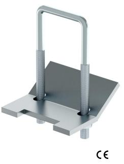
Connection element for two-sided fastening of profile rails to steel girders. Fastening is possible independently of the arrangement of the rail opening. The rail length should be at least the width of the steel girder +  $2 \times 50$  mm. Always use in pairs for mounting. For use with profile rail MS4022, MS4141, MS4142, MS4124.
