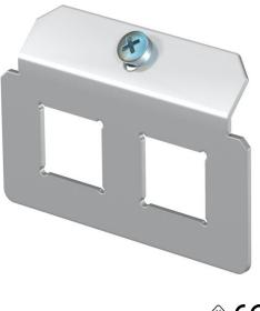
Support plate to accept two data connection modules of the following types: Lex-Com 125 and 250. Dimensions of a mounting opening in mm: 18.30 x 17.20.
