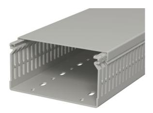
Wiring duct, incl. cover and base perforation, for horizontal and vertical routing of electrical cables in the switchgear cabinet. Designed as a metric duct. The nominal dimension of the system size corresponds to the internal dimension of the duct. Retainers are broken out without tools. The flush-floor routing of cables is possible through predetermined break points. Tapering in the side slots prevents the cables from falling out. Tested to DIN EN 50085-2-3. Special lengths on request.
