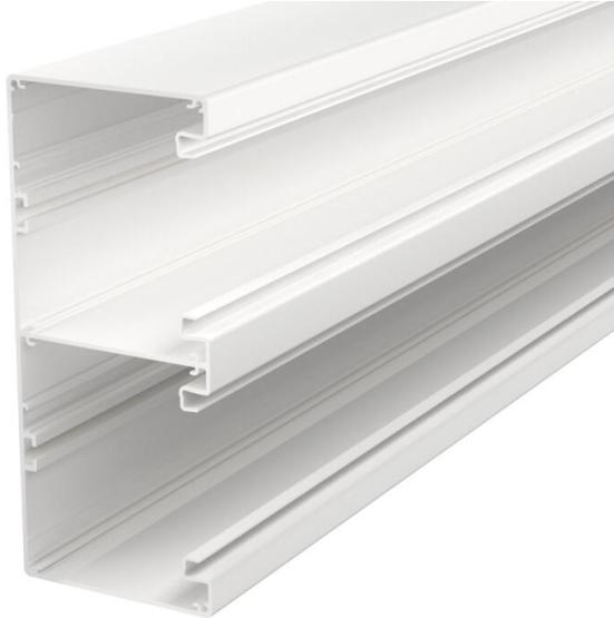
Device installation trunking Without base perforation suitable for direct wall mounting or mounting on panels. Over-lengths up to 6,000 mm for trunking bases and covers as well as other RAL colours can be provided on request. The visible surfaces of the device installation trunking are laminated.
