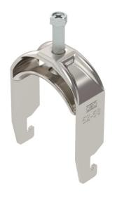
Clamp clip with U-foot, metal pressure trough with rounded edges to protect the cable. For vertical and horizontal mounting of 1 single cable on a C-profile rail. For slot width 18–22 mm. With 1-start screw thread on pressure trough, universal hexagonal screw head WAF10, with slot and cross recess. Suitable for mounting indoors and outdoors. We recommend the use of a counter-trough.
