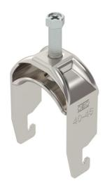
Clamp clip with U-foot, metal pressure trough with rounded edges to protect the cable. For vertical and horizontal mounting of 1 single cable on a C-profile rail. For slot width 18–22 mm. With 1-start screw thread on pressure trough, universal hexagonal screw head WAF10, with slot and cross recess. Suitable for mounting indoors and outdoors. We recommend the use of a counter-trough.
