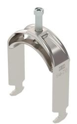
Clamp clip with hammerhead foot, metal pressure trough with rounded edges to protect the cable. For vertical and horizontal mounting of 1 single cable on a C-profile rail. For a slot width of 16–17 mm. With 1-start screw thread on pressure trough, universal hexagonal screw head WAF10, with slot and cross recess. Suitable for mounting indoors and outdoors. We recommend the use of a counter-trough.
