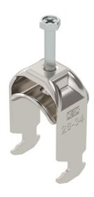
Clamp clip with hammerhead foot, metal pressure trough with rounded edges to protect the cable. For vertical and horizontal mounting of 1 single cable on a Cprofile rail. For a slot width of 16-17 mm. With 1-start screw thread on pressure trough, universal hexagonal screw head WAF10, with slot and cross recess. Suitable for mounting indoors and outdoors. We recommend the use of a countertrough.
