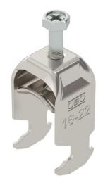
Clamp clip with hammerhead foot, metal pressure trough with rounded edges to protect the cable. For vertical and horizontal mounting of 1 single cable on a C-profile rail. For a slot width of 16–17 mm. With 1-start screw thread on pressure trough, universal hexagonal screw head WAF10, with slot and cross recess. Suitable for mounting indoors and outdoors. We recommend the use of a counter-trough.
