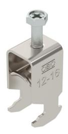
Clamp clip with hammerhead foot, metal pressure trough with rounded edges to protect the cable. For vertical and horizontal mounting of 1 single cable on a C-profile rail. For a slot width of 16–17 mm. With 1-start screw thread on pressure trough, universal hexagonal screw head WAF10, with slot and cross recess. Suitable for mounting indoors and outdoors. We recommend the use of a countertrough.
