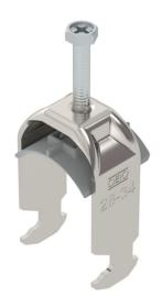
Clamp clip with hammerhead foot, plastic pressure sleeve made of polypropylene. For vertical and horizontal mounting of 1 single cable on a C-profile rail. For a slot width 16–17 mm. With 1-start screw thread on pressure sleeve, universal hexagonal screw head WAF10, with slot and cross recess. Suitable for assembly indoors and outdoors. We recommend the use of a counter-sleeve.
