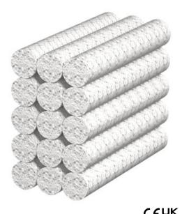
The noise limit barrier is used to reduce the transmission of airborne noise, e.g. when the trunking system is run through a wall between two offices. The noise limit barrier is made of glass wool, which, when delivered, has a diameter of approx. 30 mm and a length of approx. 300 mm. The material need not be greatly compressed during mounting.
