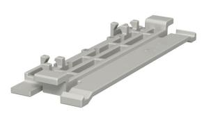
Cover clip for better and easier laying of lines in the WDK trunking. The cover fixing device can be moved along the entire length of the trunking. The cover clip is locked on one side and moved forward. This provides a 30° opening, meaning that cable routing is very simple. From trunking widths of 110 mm, the cover clips can also be used as a mounting
